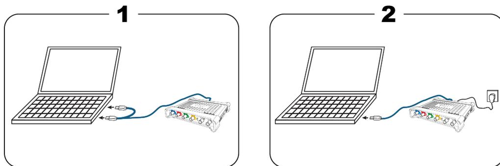
**Note:** If you connect or disconnect the AC adaptor while the oscilloscope is in operation it will restart automatically and any unsaved data will be lost.
