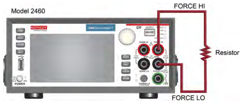
Figure 19: Model 2460 2-wire front-panel connections
