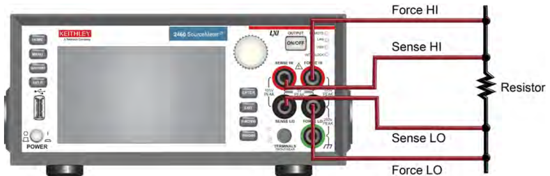
Figure 52: Model 2460 4-wire connections to the front panel
