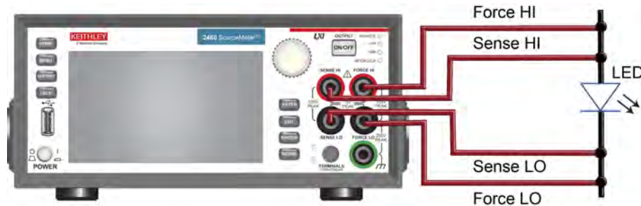
Figure 35: Model 2460 4-wire front-panel connections to an LED
