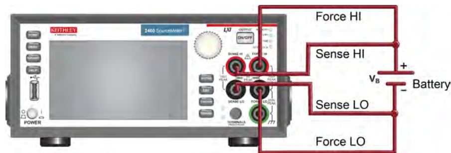
Figure 28: Front-panel connections for the battery discharge-charge application
