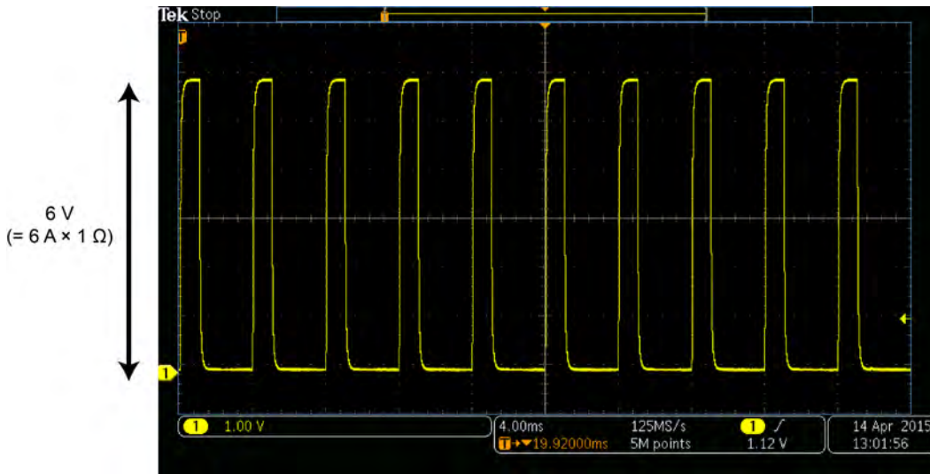
Figure 56: Oscilloscope view of ten 1 ms, 6 A pulses into a 1 Ω load with a period of 4 ms
