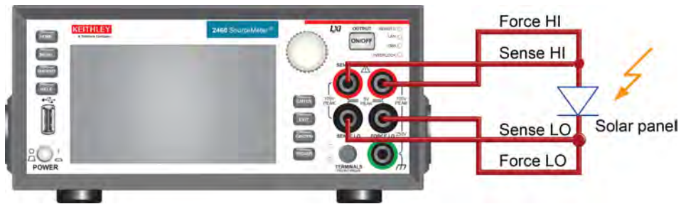
Figure 45: Model 2460 4-wire connections to the front panel
