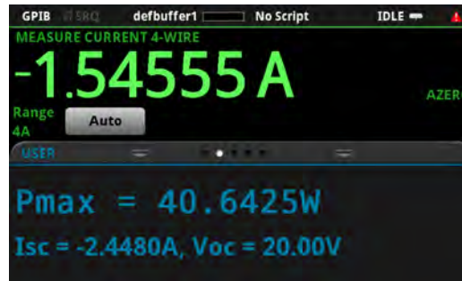
Figure 48: Solar panel I-V sweep results on the USER swipe screen
