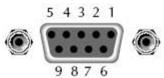
The plug pins of RS232
