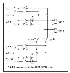
Scanner Configuration for Models 2000-SCAN and 2001-SCAN
