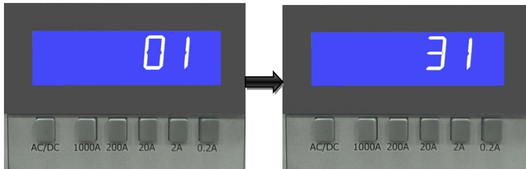
Once the required address is reached press AC/DC key to save the New Address and return to the normal screen.
