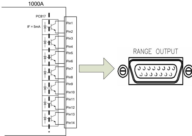
Fig 2-8 RS-232C RANGE OUTPUT CONNECTION OF REAR PANEL
