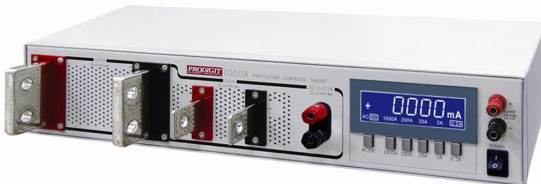
The compliance voltage of the shunt is less than 0.2 volts at full scale for each range except the 1000 Ampere range which has a compliance voltage of 0.1 volts. The shunt is a highly stable AC/DC resistor connected in a four-terminal non-inductive configuration for each range except the 1000A range.
