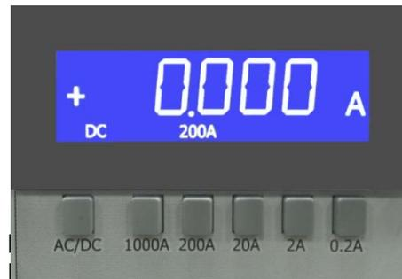
Pressing the "200A" key on the 1000A current Shunt, the appropriate LCD will
