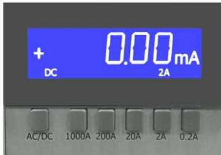
Pressing the "0.2A" key on the 1000A current Shunt, the appropriate LCD will illuminate according to the operating range is selected.
