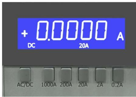
Pressing the "2A" key on the 1000A current Shunt, the appropriate LCD will illuminate according to the operating range is selected.
