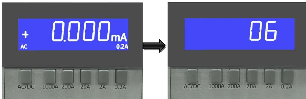
Press 2A (UP), 20A (down) buttons to adjust the GPIB address 1 to 31.
