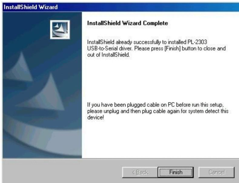
2. After the installation, connect the 1000A and PC with USB. Then select the item USB to Serial Port (COM3), set the BAUD-RATE to 115200bps and the Flow control to Hardware. You should then be able to control the 1000A via USB on COM3.
