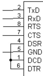
Fig 4-1 RS-232C INTERFACE CONNECTION OF REAR PANEL
