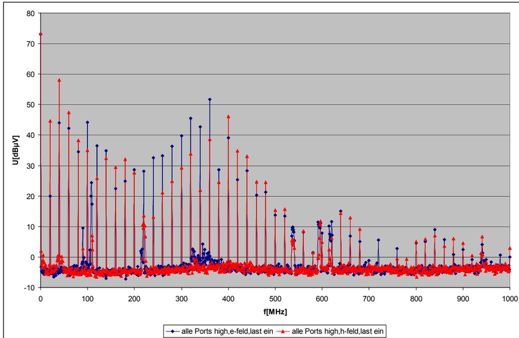
Figure 3.2: Effect of the RF bypass on the emission of disturbances
