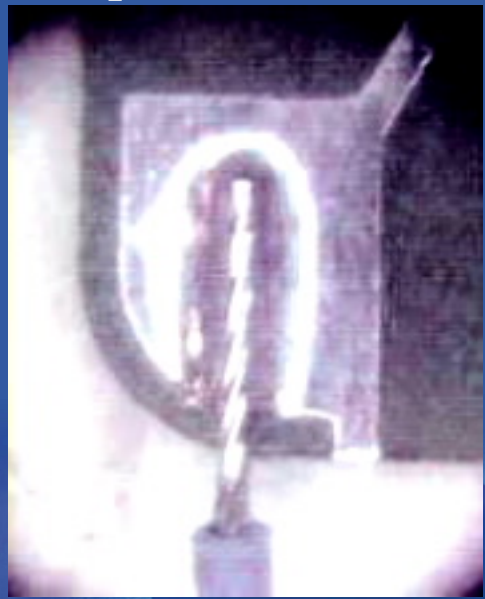
普通焊丝例子 Good sample of Sn60
