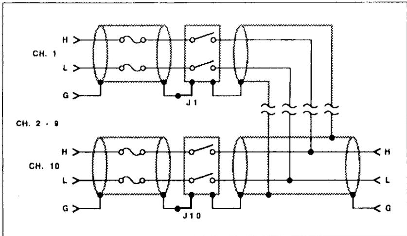
**Figure 1-1. Model 7154 Simplified Schematic**
