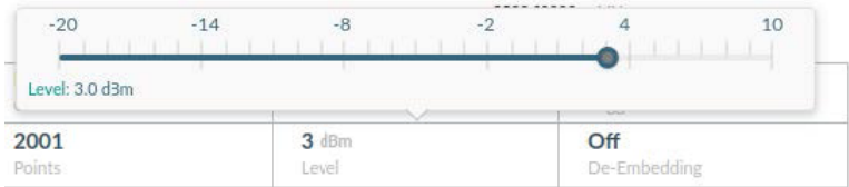
Figure 6.5.2: Setting the test signal level, via the popup located below the main display.
