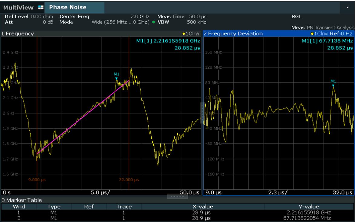
Analysis of linearity of FMCW chirps. Left: the pink reference line can be seen between the evaluation lines. Right: the deviation of the frequency from linear behavior is displayed.
