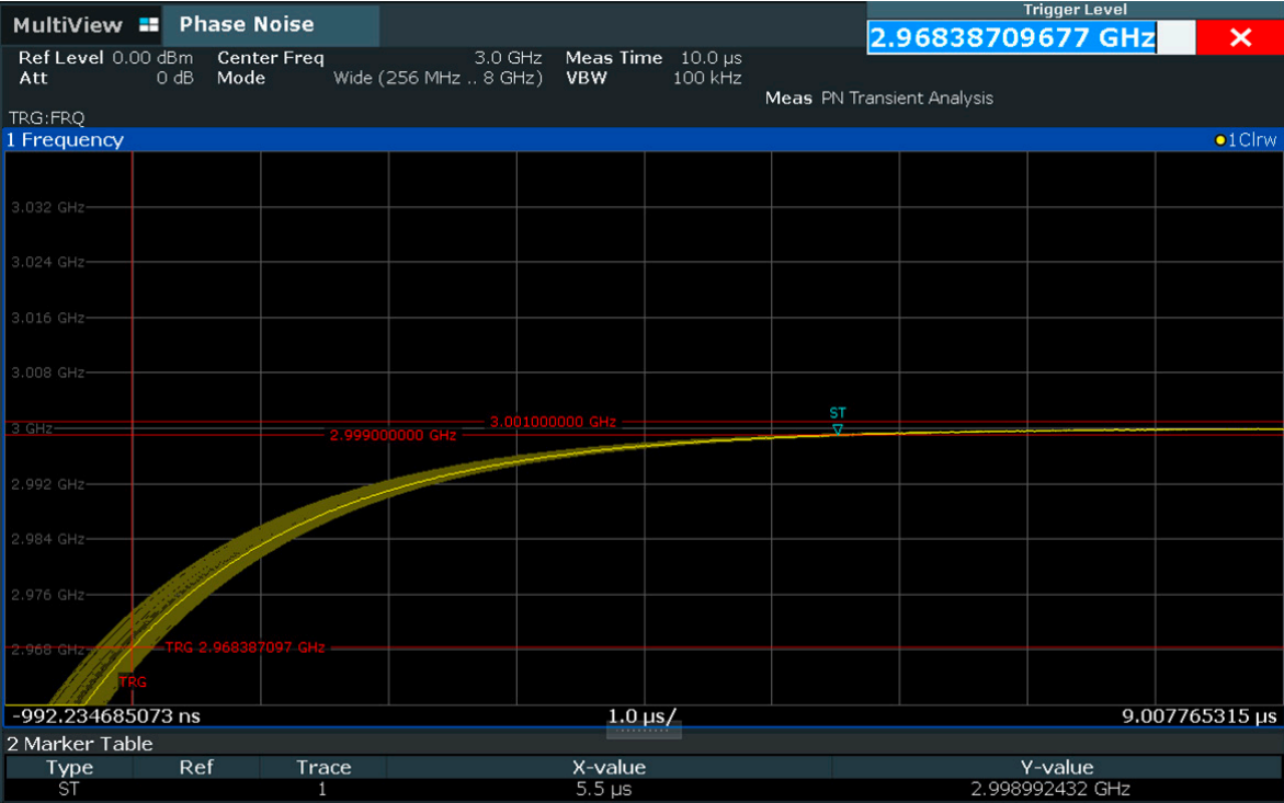
Transient response of a synthesizer in persistence mode. The horizontal red line shows the frequency trigger threshold, the vertical line the trigger offset. The bright yellow trace is the current measurement, the dull yellow traces show all previous measurements.
