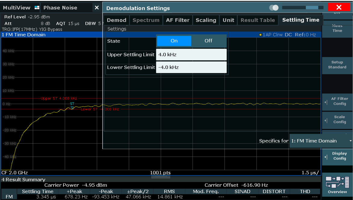
Automatic settling time measurement: after defining the tolerance frequency range the settling time is displayed in the result summary.
