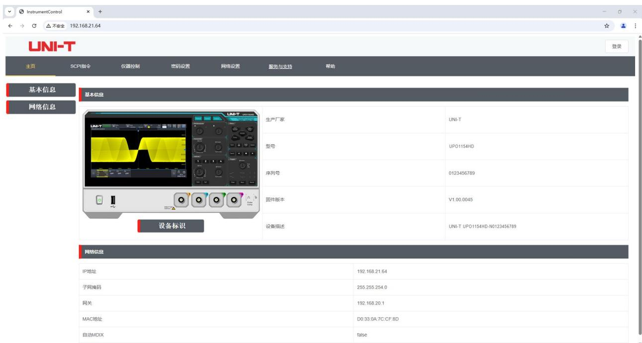
The screenshot shows a web browser window with the address bar displaying 'InstrumentControl' and '192.168.21.64'. The page title is 'UNI-T'. The navigation menu includes '主页', 'SCPI指令', '仪器控制', '密码设置', '网络设置', '服务与支持', and '帮助'. The main content area is divided into two sections: '基本信息' (Basic Information) and '网络信息' (Network Information). The '基本信息' section displays a device image and a table of details:
