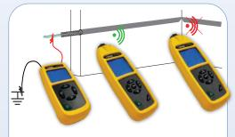
Detect the narrowed (or blocked) section of a non-metallic pipe (requires temporary insertion of a conductor)
