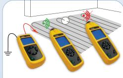
Detect faults in an underfloor heating system (unshielded resistance)
