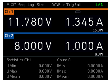
Figure 5-6: Fuse indicator display at channel 1
