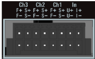
Figure 3-7: Terminal block with connector assignment
