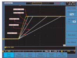
The Adjustable Rise Time of the PSW 800V Module
