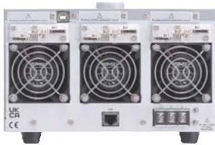
Three-channel Models Rear Panel
