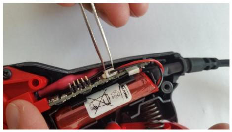
■ Lift the storage battery clear and unclip it.
