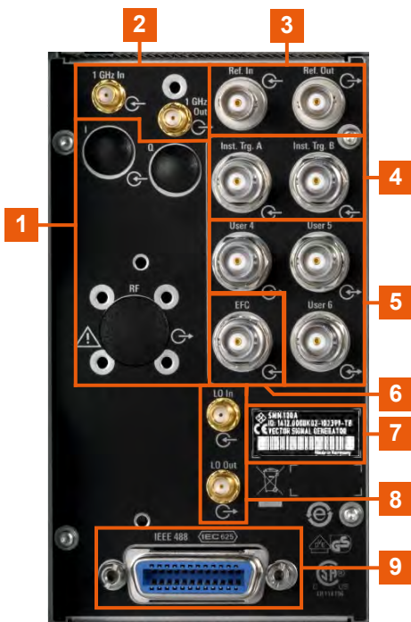
Figure 4-4: Connectors for rack use, external reference signal, external frequency control, local oscillator and remote control
