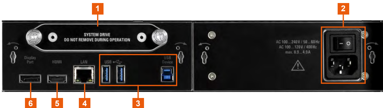
Figure 3-6: System drive, power switch, power supply, monitor, LAN and USB connectors
