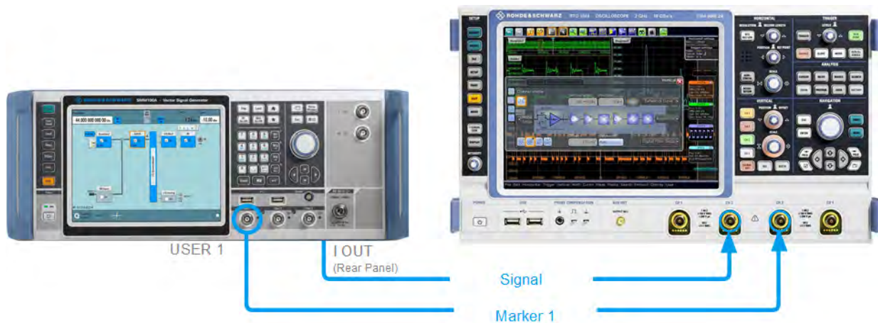
Figure 3-14: Simplified representation of a test setup for signal monitoring**
