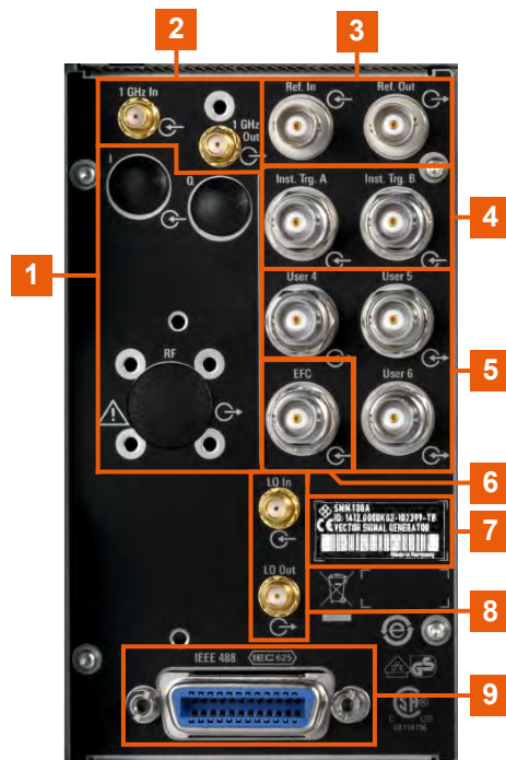
Figure 3-5: Connectors for rack use, external reference signal, external frequency control, local oscillator and remote control
