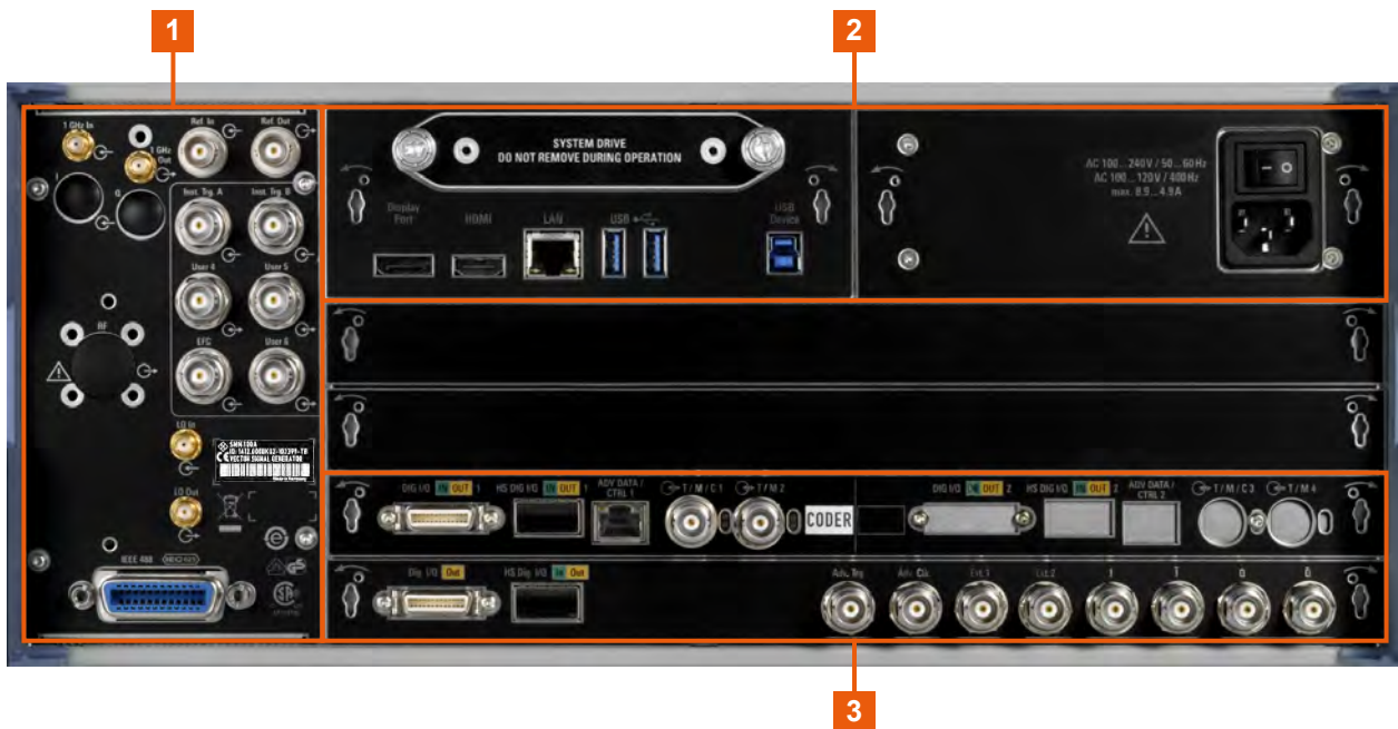
Figure 3-4: R&S SMM100A rear panel controls and connectors (R&S SMM-B9)
