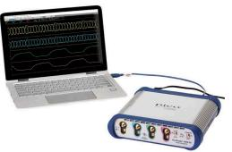
4-channel, 12-bit, 5 and 16 GHz samplerextended real-time oscilloscopes. Capture pulse and step transitions down to 22 ps and clocks and data eyes to 8 Gb/s.
