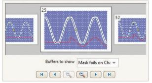
Up to 10 000 waveforms can be stored in the segmented waveform buffer. The Buffer Overview window then allows you to rewind and review the history of your waveform.
