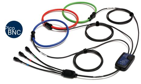
The TA325 is a switched-range 30/300/3000 A AC RMS probe with 10 Hz to 20 kHz bandwidth, rated to 1000 V CAT III on uninsulated conductors. Suitable for measuring 3-phase AC current, it has three sensor coils and scope connection leads, color-coded to match Channels A, B and C in the PicoScope software. Typical battery life is 1000 hours.
