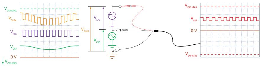
Differential scopes can measure the AC or DC voltage between two points connected to the positive and negative leads, when neither of the points is grounded. This enables them to take measurements where single-ended scopes can't, for example at voltages that are much higher than ground potential. The resulting measurements focus exclusively on the potential difference between the probes.
