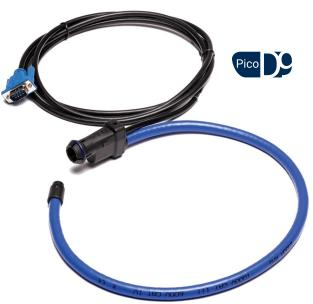
The TA368 is a 2000 A AC RMS probe with 10 Hz to 20 kHz bandwidth, rated to 1000 V CAT III and 600 V CAT IV on uninsulated conductors. It has a flexible sensor coil, enabling you to measure currents on hard-to-reach conductors.
