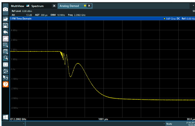
Frequency settling behavior of an oscillator
