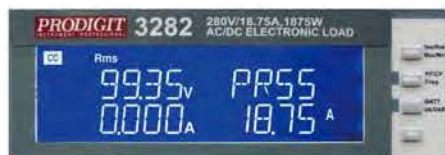
Turbo OFF, Short 100mS 18.75A Test result
