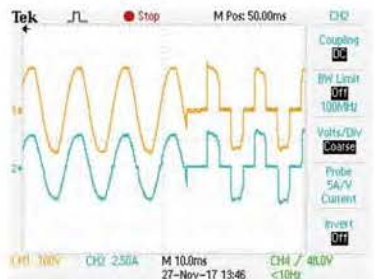
Linear CC mode, UPS Sine to Square waveform
