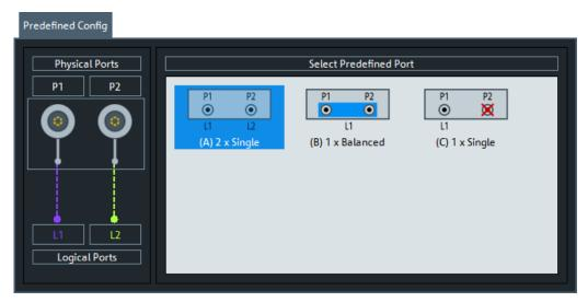
The port configurations are arranged in the list to the right. The resulting port assignment is shown on the left-hand side of the "Predefined Config" tab.
