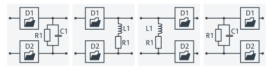
The following networks are composed of two serial Cs or Ls (as seen from the analyzer test port), followed by a shunt C or L. They are named Serial Cs, Shunt L / Serial Ls, Shunt C / Serial Ls, Shunt L.
