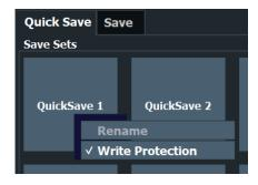
During recall, save sets of type "Instrument" replace the settings of the entire instrument. All other save sets start a new channel setup with the stored settings.
