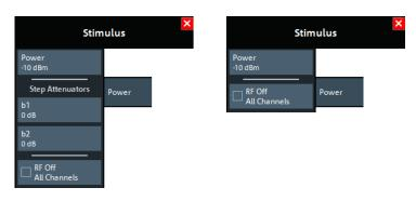
left = R&S ZNL with Receiver Step Attenuators right = R&S ZNLE (or R&S ZNL without receiver step attenuators)
