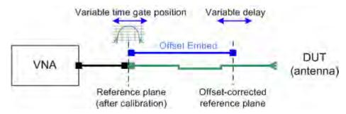
If "Adjust Time Gate" is on, the time gate is moved to left (right) when the offset-corrected reference plane is moved to the right (left). Its absolute position remains fixed. With this setting, it is possible, e.g., to keep the time gate at the position of the antenna connector while the antenna is measured at different length offsets.
