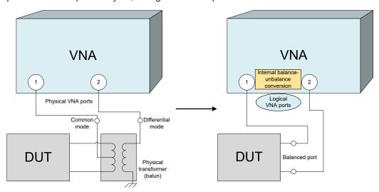
Unbalance-balance conversion avoids the disadvantages of real transformers:
