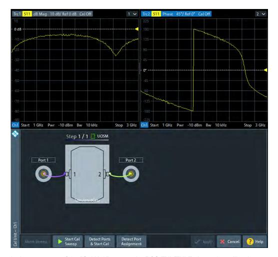
In the upper part of the "Cal Unit" screen, the R&S ZNL/ZNLE shows the calibration sweep diagrams for the currently measured S-parameter. The lower part visualizes the active port assignment and the measurement progress.
