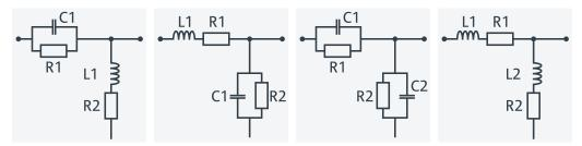
The following networks are composed of a shunt C or L (as seen from the analyzer port), followed by a serial C or L. They are named Shunt C, Serial L / Shunt L, Serial C / Shunt L, Serial L.
