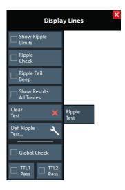
The "Def. Ripple Test..." button opens the "Define Ripple Test" dialog (see Chapter 10.9.5.2, "Define Ripple Test Dialog", on page 422).
