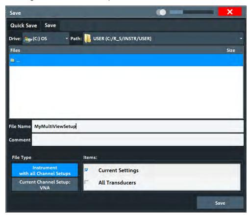
Figure 4-7: Saving the instrument settings to a file
