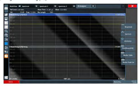
Figure 4-9: Inserting a Real/Imag diagram for I/Q analysis
