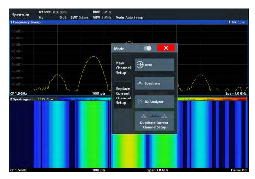
Figure 4-8: Adding a new channel setup
