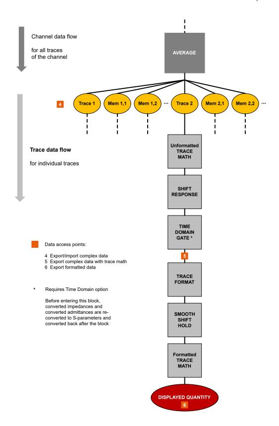
This section describes manual operation of the VNA mode, including trace settings, markers and diagrams. For a description of the different quantities measured by the instrument, refer to Chapter 9.3, "Measurement Results", on page 217.
