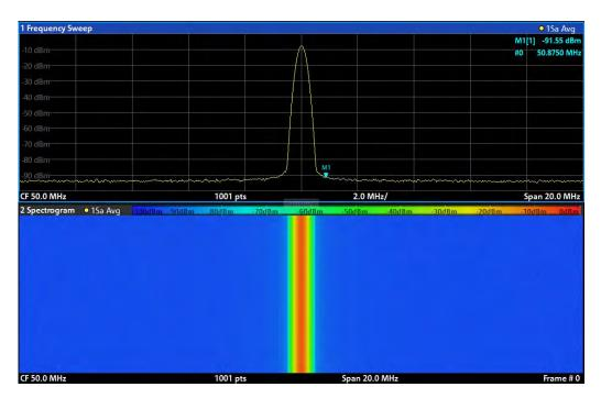
Figure 4-14: Spectrogram of the calibration signal
