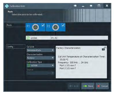
Figure 10-11: Calibration Unit wizard, step 1: Ports
