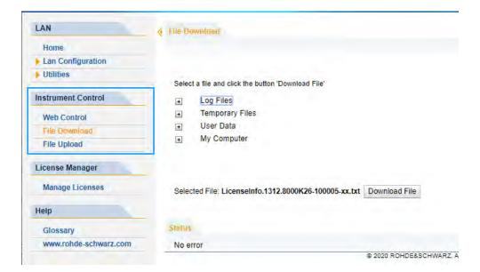
The most commonly used folders on the instrument are displayed, for example those that contain user data, as well as the top-most My Computer folder, from which you can access all other folders on the instrument.
