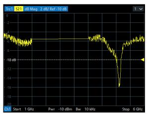
**Tip:** You can change to point based x-axis to improve the display of a segmented frequency sweep (see "Seg X-Axis" on page 316).
