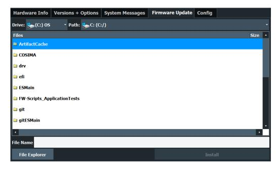
Enter the name or browse for the firmware installation file and press the "Install" button.
