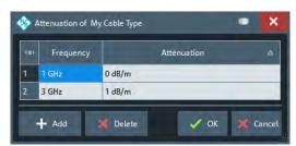
Given the specified attenuation values the R&S ZNL/ZNLE calculates the attenuation factor at the center of the channel's sweep range and corrects the impulse response trace using this attenuation factor Attenuation ( $f_{center}$ ).
