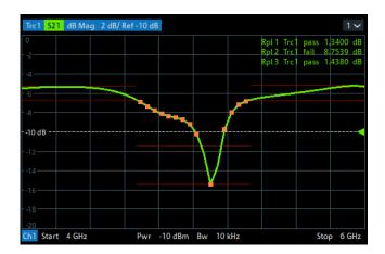
The limit line rules for logarithmic sweeps and segmented frequency sweeps with point-based x-axis also apply to ripple limit lines (see Chapter 9.4.1.1, "Rules for Limit Line Definition", on page 232).
