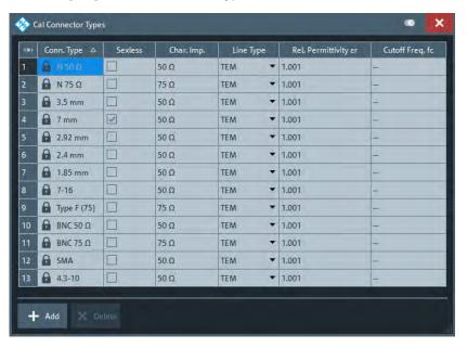
The list shows the available connector types with their name ("Conn. Type") and polarity ("Sexless"). The remaining columns in the list are described below.
