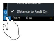
"Distance to Fault" can also be enabled/disabled via the context menu of the trace label.
