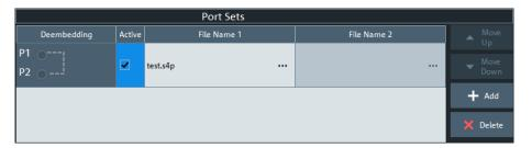
The "Port Sets" panel can also be activated by selecting the Port Sets Tab. Refer to its description for background information, parameters and additional remote commands.
