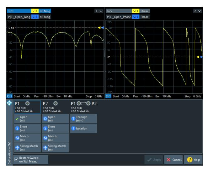
Figure 10-14: Calibration Setting Wizard, Step 3: Calibration
