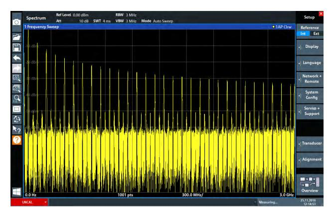
Figure 4-12: Calibration signal with optimized display settings
