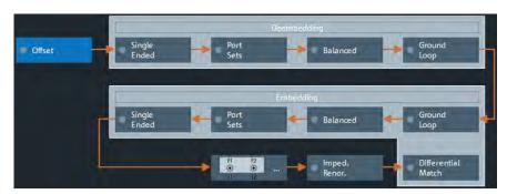
Figure 9-5: De-/Embedding calculation flow
