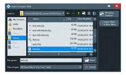
On loading data from a trace file with several traces, the analyzer displays a dialog to select one or more of the traces stored in the file (see Chapter 10.6.11.3, "Select Parameter Dialog", on page 373). E.g., for an \*.s2p Touchstone file, the box offers all four 2-port S-parameters (see Chapter 9.4.2.1, "Touchstone Files", on page 239).
