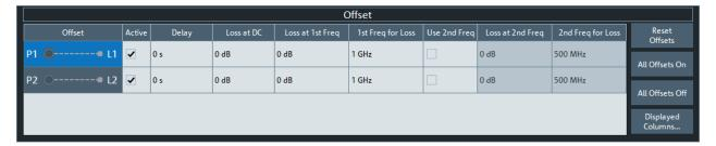
Figure 10-18: Offset Embed dock widget: Offset panel
