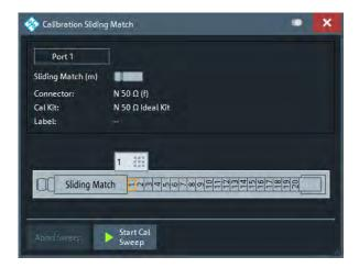
Figure 9-3: Sliding Match: GUI representation
