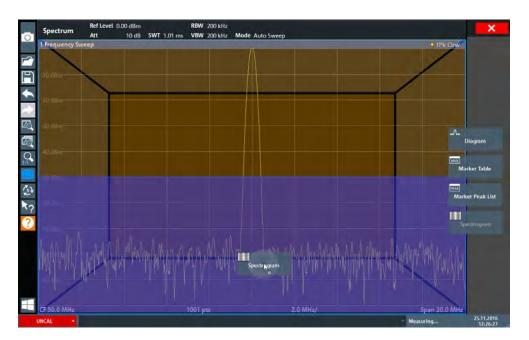
Figure 4-13: Adding a Spectrogram to the display
