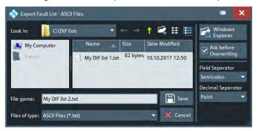
This CSV type file contains one line (terminated by CR+LF) per fault. With ";" as "Field Separator" and "." as "Decimal Separator", the fault list of Figure 10-4 is exported to
