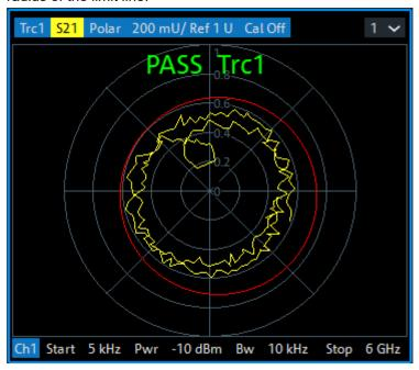
With a circle limit line adjusted to the right border of a Smith diagram (Z = infinity), you can check whether the imaginary part of the impedance (Im(Z), reactance) falls below a limit.
