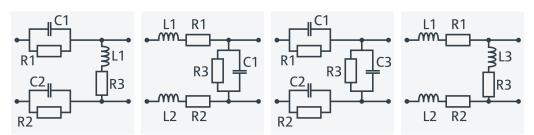
The following networks are composed of a shunt C or L (as seen from the analyzer test port), followed by two serial Cs or Ls. They are named Shunt L, Serial Cs / Shunt C, Serial Ls / Shunt C, Serial Cs / Shunt L, Serial Ls.
