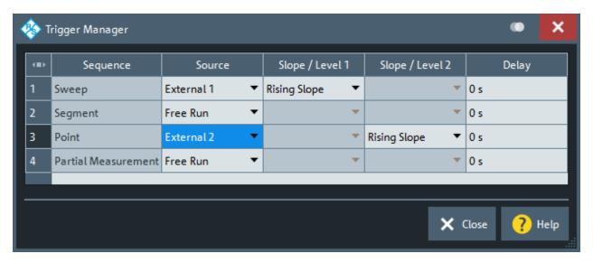
Figure 10-3: Example of a multiple trigger configuration
