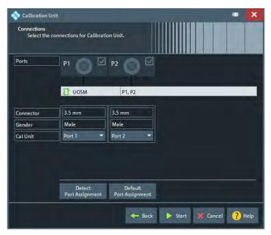
Figure 10-12: Calibration Unit wizard, step 2: Connections
