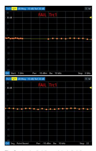
**Tip:** Overlapping limit line and ripple limit line segments are not displayed when a point-based x-axis is active; see Chapter 9.4.1.1, "Rules for Limit Line Definition", on page 232.
