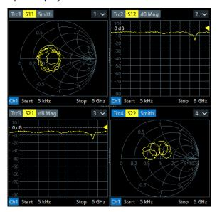
If less than two (three / four) traces are available, the new diagrams are created with a default trace. Dual (triple / quad) split corresponds to "Split Type: Tile Horizontal" with 2(3/4) diagrams.
