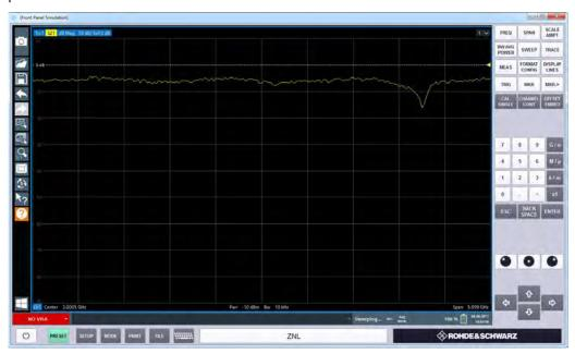
To activate or deactivate the front panel temporarily, press the [F6] key on the external keyboard (if available) or the remote computer.
