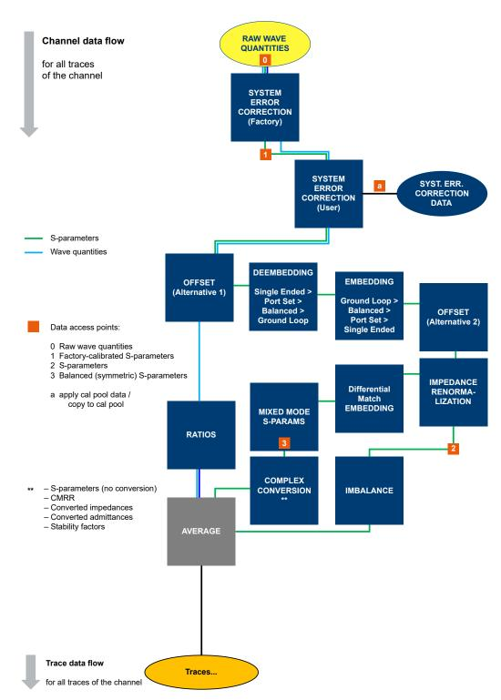
Figure 9-1: Channel data flow
