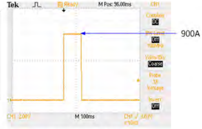
3356G Turbo mode ON Short real test waveform
