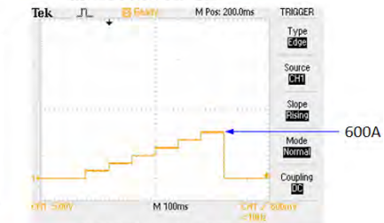
3356G Turbo mode OFF OCP Istep 10A, Istop 600A real test waveform
