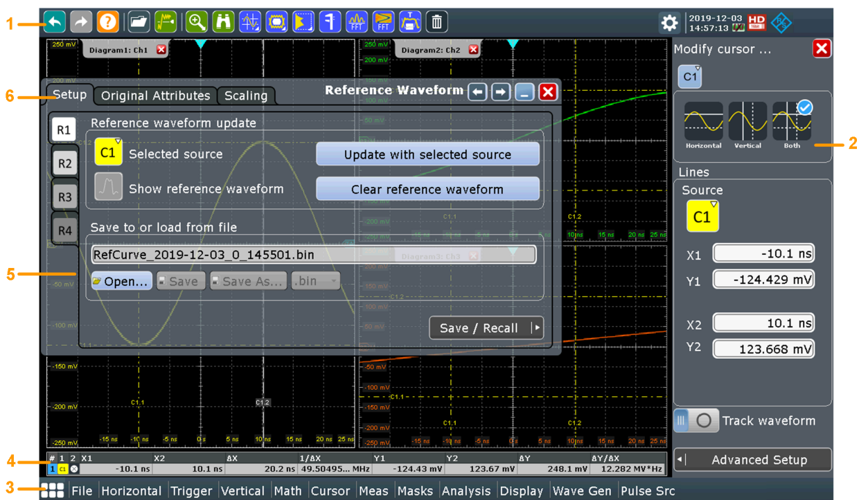
Figure 6-4: Control elements on the touchscreen
