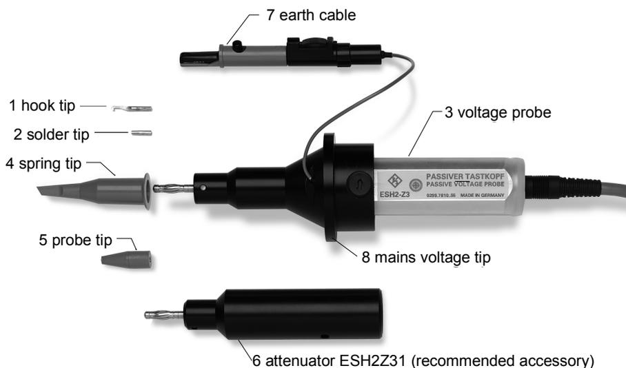
For disturbance voltage measurements in the frequency range 9 kHz to 30 MHz ground connection of the probe is very important. It is to be established by connecting the earth cable **7** to the RF ground of the item under test.
