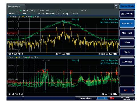
Upper part of screen: continuous spectral display of RF input signal around the current receive frequency using the IF analysis function. Lower part of screen: stored results of preview measurement. The center frequency in the upper diagram is controlled by the marker position in the lower diagram (marker track function). Alternatively, the IF spectrum display can be coupled with the combined numeric and bargraph display.
