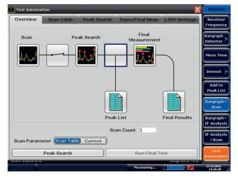
The R&S°ESRP allows users to configure automatic test sequences (preview measurement, data reduction, final measurement) quickly and easily and execute them at the press of a button. The final measurement can also be carried out interactively.
