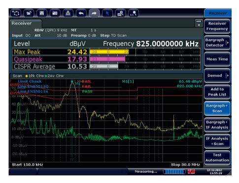
The R&S°ESRP performs disturbance voltage measurements with quasi-peak and average weighting in a matter of seconds.
