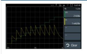
In this example, the charging current of a capacitor is displayed while the voltage is increased stepwise.
