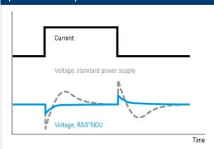
Under challenging load conditions, most power supplies respond with slow recovery times and overshoot. Specially developed circuits in the R&S®NGU source measure units achieve a load recovery time of < 30 µs with minimal overshoot, making them perfect for supplying sensitive components with power.
