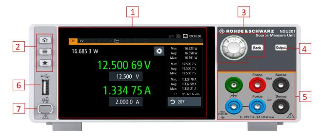
Figure 4-1: Front panel of NGU201 model
