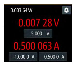
Figure 6-2: Output of R&S NGU in CC mode
