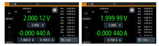
Figure 6-8: NGU201 model switches from VPM to CPM
