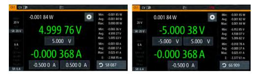
Figure 6-9: NGU401 model switches from VPM to CPM
