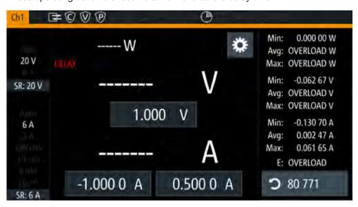
Figure 6-7: Delay text at channel display area
