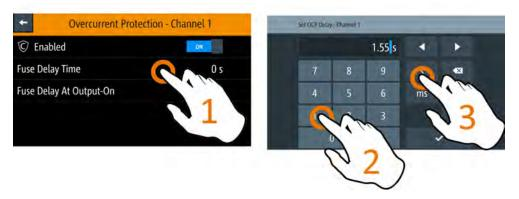
Figure 5-6: Enter numerical value and unit
