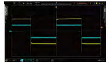
Linear CC mode, PWM 10A 250Hz
