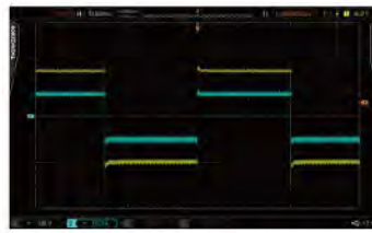
Linear CC mode, PWM 10A 2.5Hz
