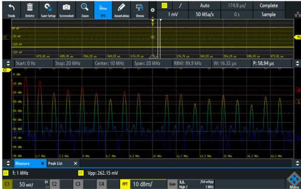
Time, frequency and protocol information are correlated, and time references can be quickly recognized. Measurement windows help you select specific areas of the recording, which can simplify, for example, the acquisition of frequency switching operations.
