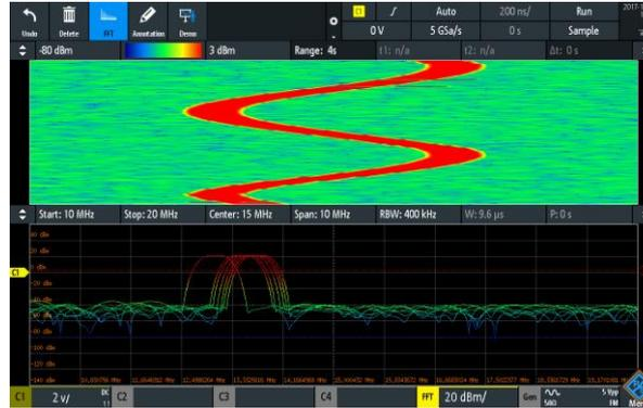
A spectrogram displays the spectrum of frequencies as they vary over time. For easy interpretation, the magnitude can be color-coded. Thanks to the high FFT rate, even fast frequency changes can be displayed.
