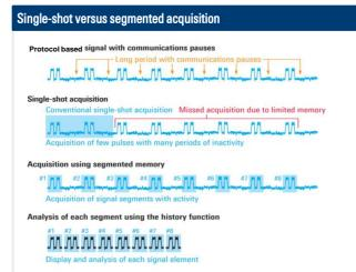
Long data sequences are usually acquired in a seamless single shot. With a maximum record length of only a few milliseconds, acquisition is often limited to a single event or protocol packet. The memory can be divided into several steps. When the fast segmented memory mode is activated, the blind time is reduced to 0.5 µs.
