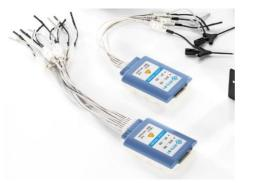
The digital inputs are grouped into logic probes with eight channels. High input impedance combined with low input capacitance of 100 k $\!\Omega$  II 4 pf ensures high signal fidelity and low loading of the test points.
