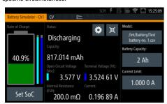
The charging behavior of a battery can also be simulated, for example when designing battery chargers. In this application, the R&S®NGM200 is used in sink mode.
