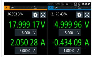
The linear design of the output stages reduces residual ripple and noise to a minimum and makes them perfect for the development of power amplifiers and MMICs.
