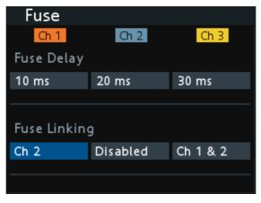
Users can set the power supply so that all channels are switched off if one channel hits the limit. Or it can be set to leave one channel working.
