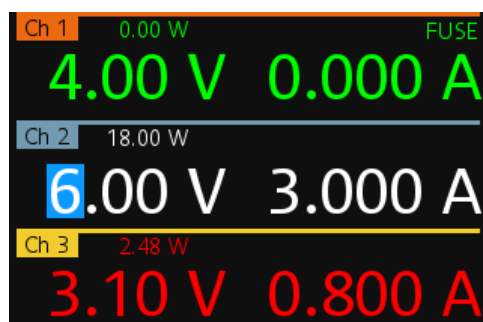
Figure 5-3: Color coding of operating condition
