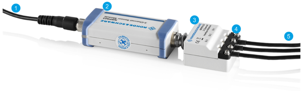
Figure 3-4: R&S NRPM-Z3 connected to R&S NRPM3
