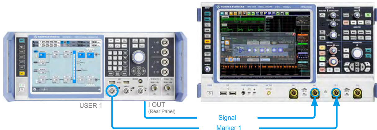
Figure 6-7: Simplified representation of a test setup for signal monitoring**
