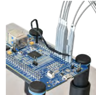
When you find a header with signals situated together and not enough grounds. A ground lead can be used to connect to a remote ground pin on the device under test.
