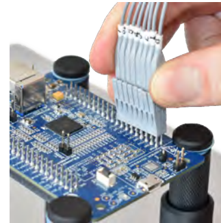
When a header has signal pins on one row and grounds on the other row.
