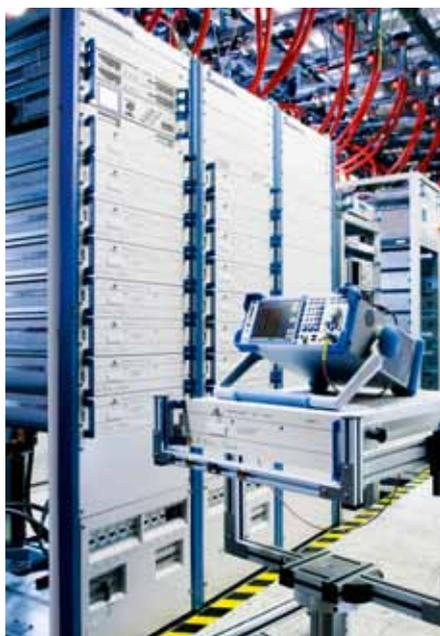
TV transmitter testing with the R&S®ETL.
