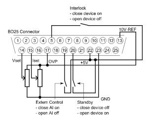
All digital outputs are OC outputs with a pull-up resistance after + 5 V. All analog inputs and outputs can be operated in 0-5 V or in 0-10 V mode.
