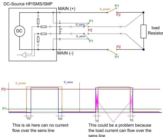
The circuit breaker ( $S_{power}$ ) must be closed when starting before the Sens ( $S_{sens}$ ). When switching off, the Sens must first be opened and then the circuit breaker can be opened. Otherwise, a current flow may occur across the sensing line, and this may be particularly critical when disconnecting.
