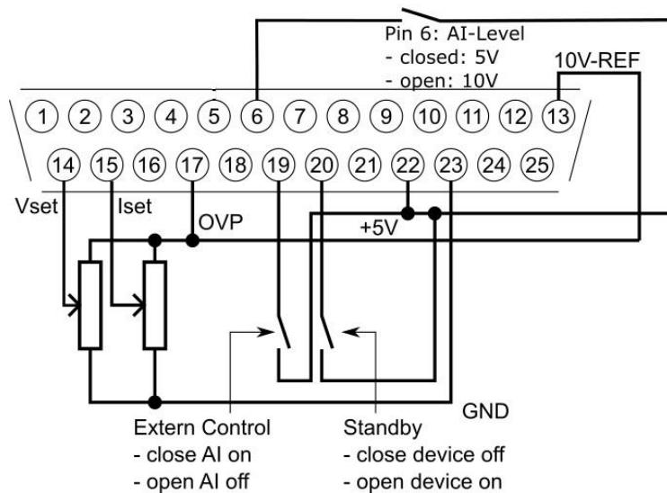
All digital outputs are OC outputs with a pull-up resistance after + 5 V. All analog inputs and outputs can be operated in 0-5 V or in 0-10 V mode.
