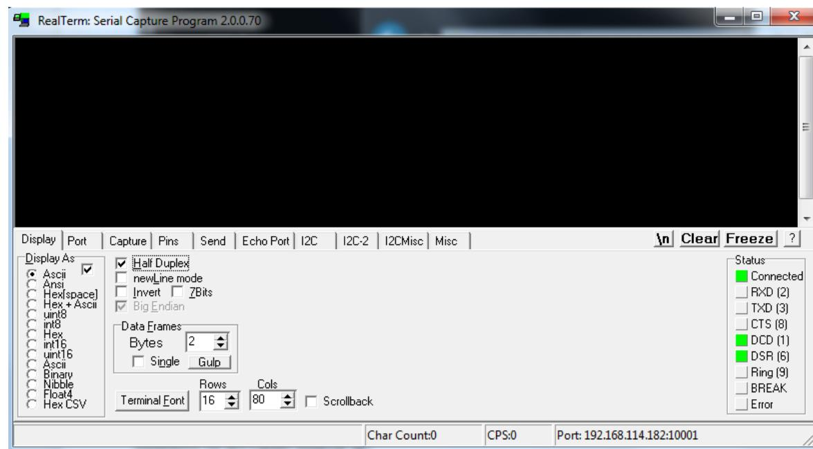
The IP address must be entered within the tab **Port** in the following format: xxx.xxx.xxx.xxx:10001. Afterwards the button **Open** must be clicked. In the terminal box the desired commands can be sent to the device.
