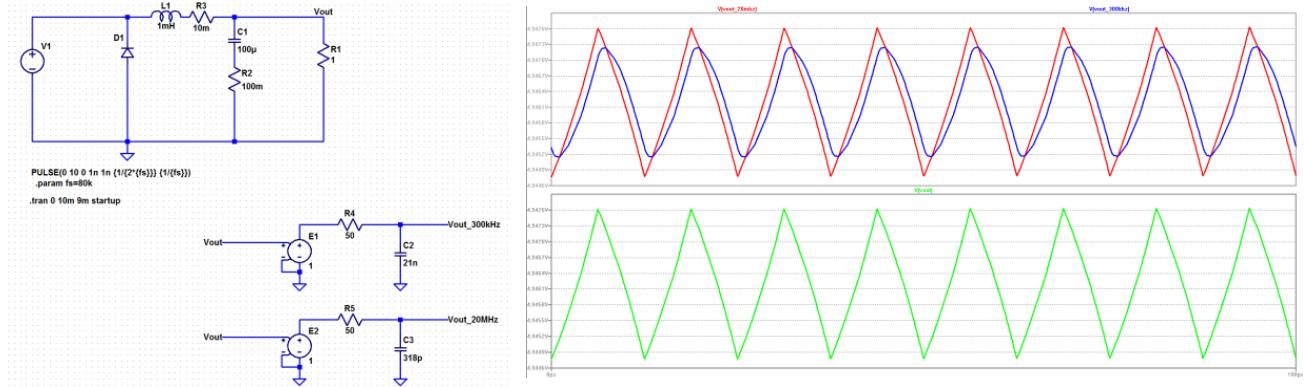
Picture 2 show the ripple without spikes. Picture 2 shows also the different between the used measurement bandwidth. At this example the switching frequency of the converter was 80kHz (this is also the switching frequency of the LAB/HP and LAB/SMS series).The red line shows the measured ripple by using a bandwidth of 20MHz and the blue line shows the measured ripple by using a measure bandwidth of 300kHz.
