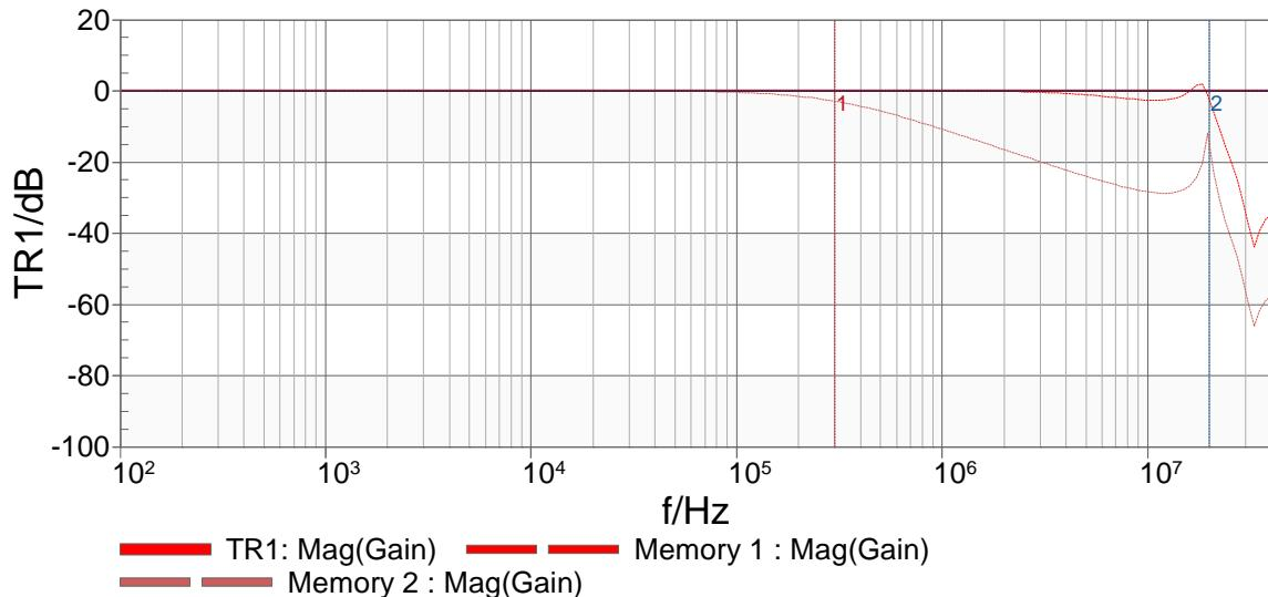
The bode plot shows that the transfer function of this circuit is very linear. This allowed making a clean and real measurement of the output ripple of a power supply also at high voltage devices.
