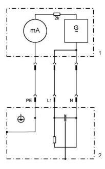
Note: The illustration shows the measurement method for two-phase power supplies. In the three-phase version, phase N is replaced by L2 and/or L3.
