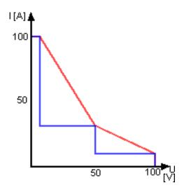
If output voltage or output current is changed afterwards, the characteristic keeps its course. Though values are stretched or compressed to the new range.
