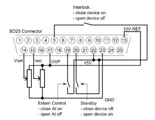
All digital outputs are OC outputs with a pull-up resistance after + 5 V. All analog inputs and outputs can be operated in 0-5 V or in 0-10 V mode.
