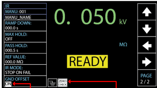
GND OFFSET cursor ZERO CHECK indicator
