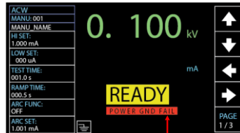
POWER GND FAIL Message
