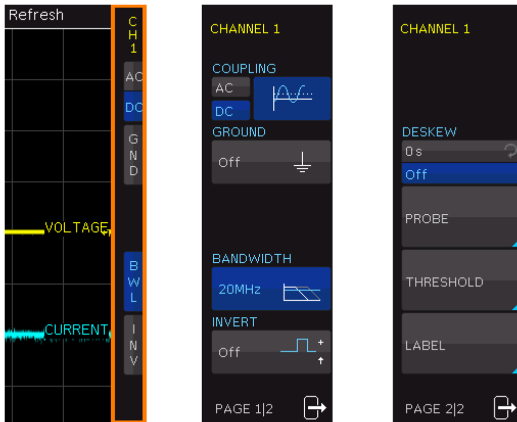
Figure 4-2: Vertical menus: short menu (left), page 1 and page 2 of the advanced menu
