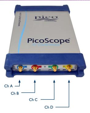
The four SMA input connections on the front of the PicoScope 6407 Digitizer allow four signals to be sampled. Various attenuators can be fitted to these connections to allow a wider range of signals to be measured on the device.
