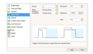
Digital triggering also reduces rearm delay and this, combined with the segmented memory, allows the triggering and capture of events that happen in rapid sequence. At the fastest timebase you can use rapid triggering to collect 10 000 waveforms in under 6 milliseconds. The mask limit testing function can then scan through these waveforms to highlight any failed waveforms for viewing in the waveform buffer.
