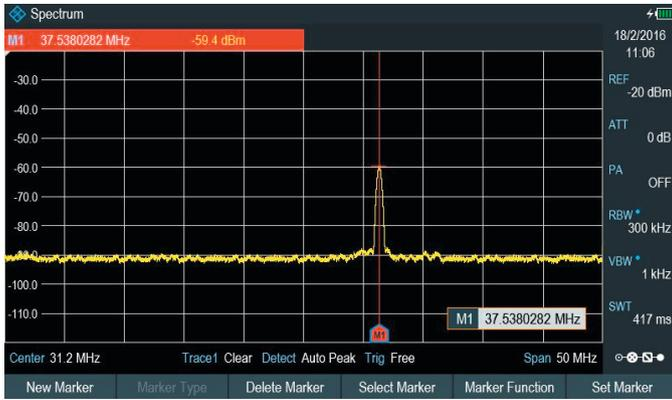
The DUT is switched off. The environmental EMI spectrum with an interferer at 37.538 MHz is measured and stored in the trace memory.
