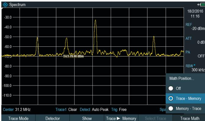
EMI spectrum of DUT with subtracted interferer. The trace math function subtracts the stored environmental EMI from the last measurement, and the R&S® Spectrum Rider displays the resulting EMI behavior of the DUT.
