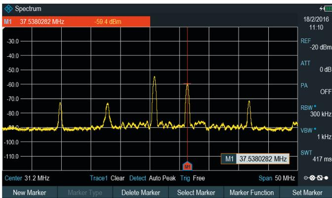
The DUT is switched on. The R&S® Spectrum Rider measures the EMI spectrum of the DUT and the environment.
