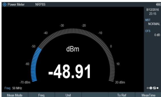
Power measurement with the R&S®NRP8S power sensor
