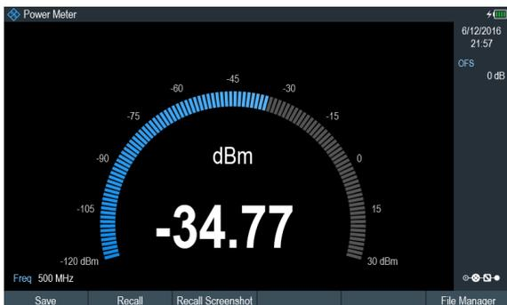
Power measurement using the internal power meter
