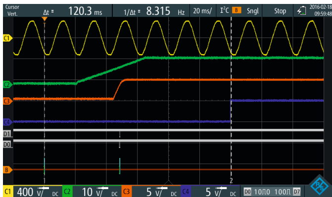
Ramp-up of an embedded AC/DC converter, programmed by PMBus/I 2 C command
