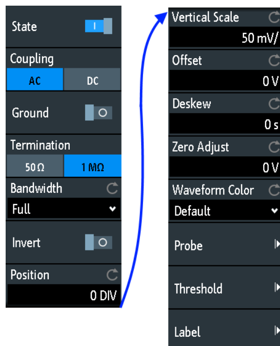
Figure 4-2: Channel menu, split into two halves
