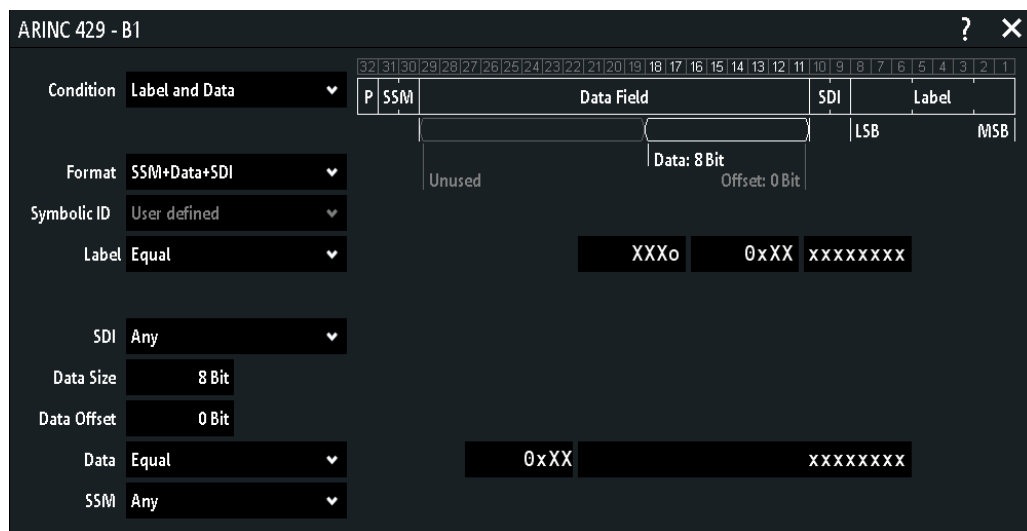
Figure 12-47: Settings for search on ARINC 429 bus
