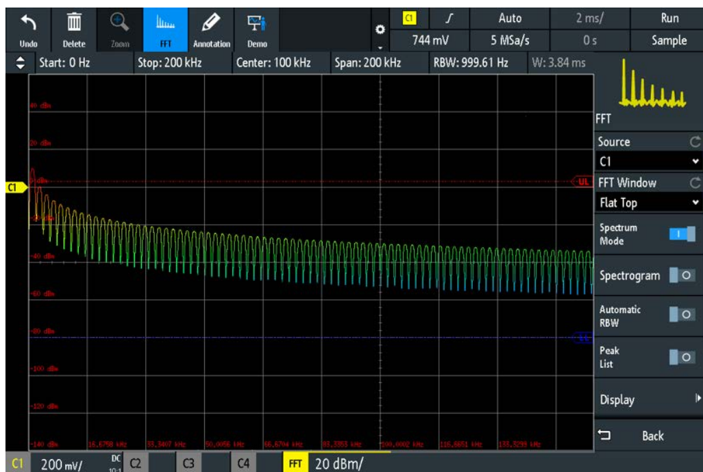
Figure 8-1: FFT display in spectrum mode
